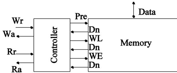
The SI controller uses **completion detection in SRAM** and handshake protocols to manage pre-charge, WL and WE in the SRAM banks
