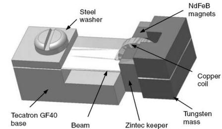
S P Beeby et al., 2007, "A micro electromagnetic generator for vibration energy harvesting", J. Micromech. Microeng. 17 (2007) 1257–1265.
