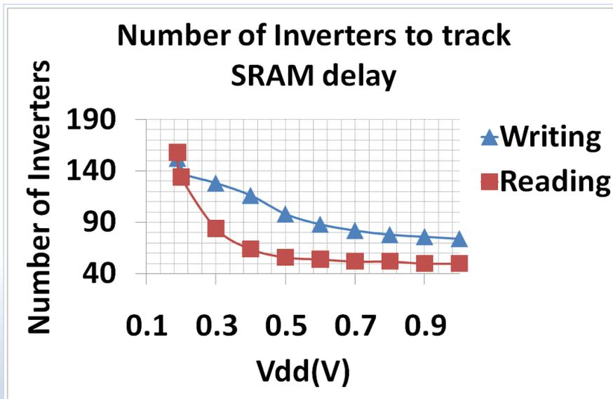
For example, under 1V Vdd, the delay of SRAM reading is equal to 50 inverters and under 190mV, the delay is equal to 158 inverters
