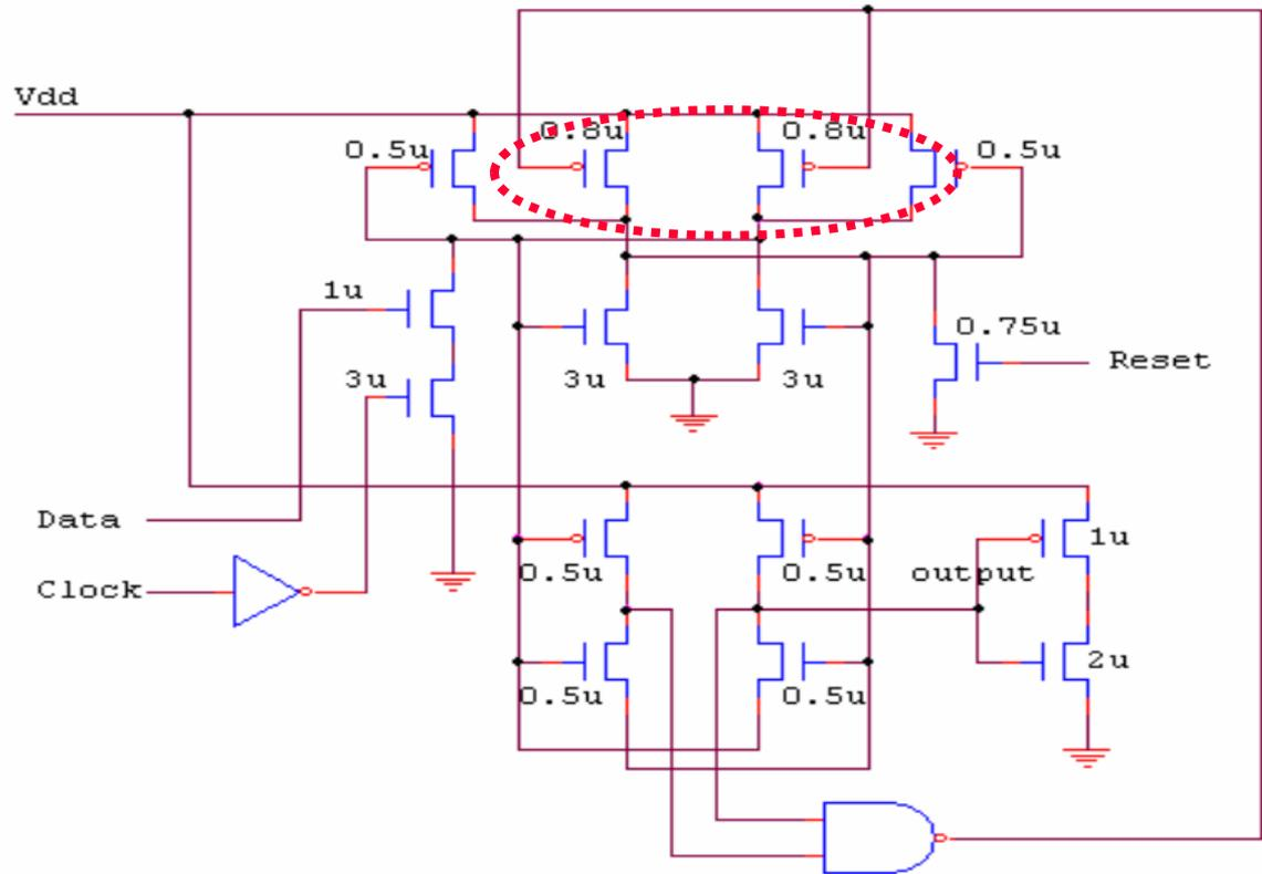
Can be further improved, to enable work at subthreshold Vdd, by means of body biasing of all main transistors
