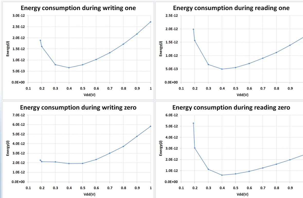
The curves show that the minimum energy point of the chip is at 400mV-500mV.
