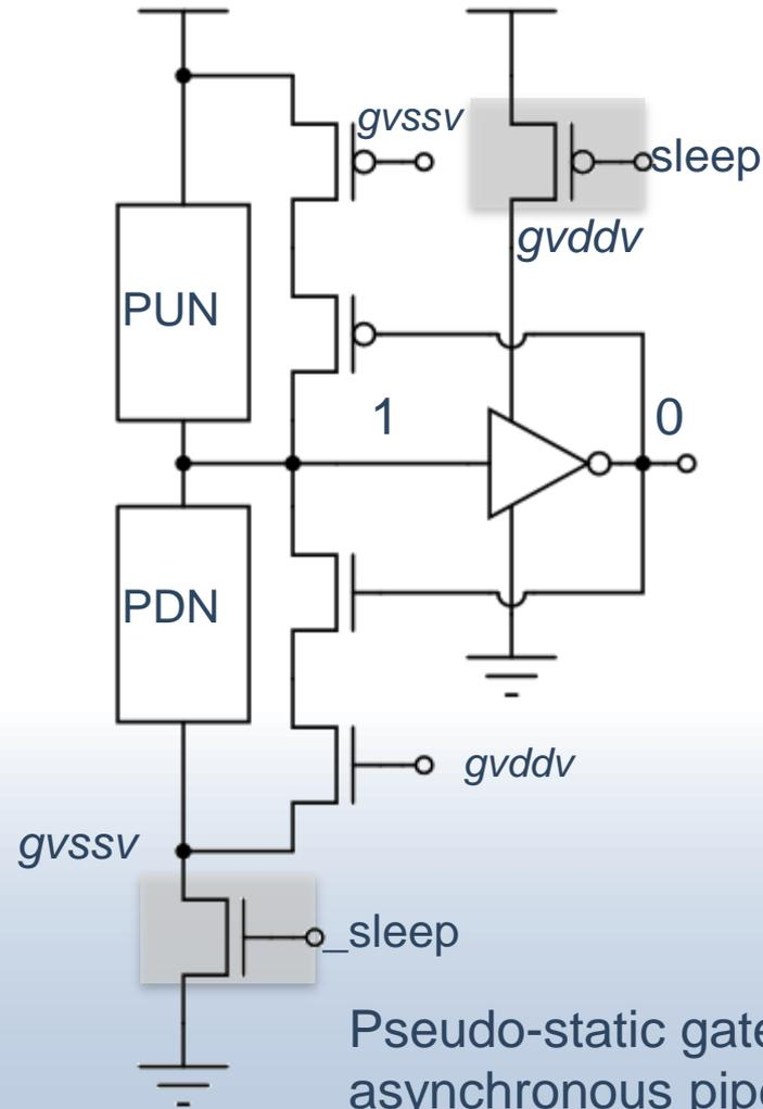
Pseudo-static gates for asynchronous pipelines
