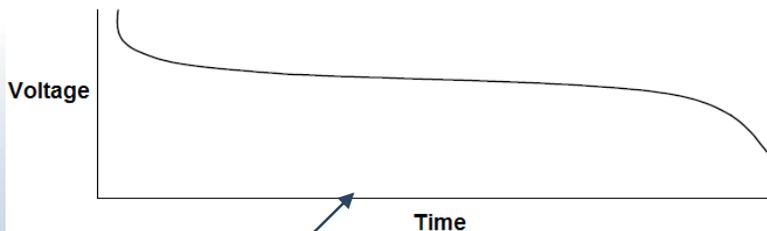
Typical Battery Discharge Curve
